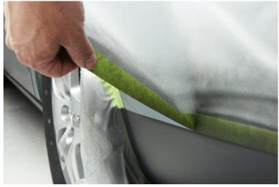
Green backing improves visibility and accuracy during paint masking
