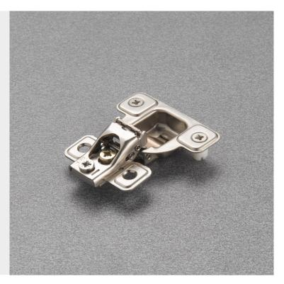
Stamped steel. Cup depth 11 mm (7/16"). Opening 106° degrees. Drilling distance (K) fixed at 2.5 mm (3/32"). Gap between door and frame (L) = 4.6 mm.
