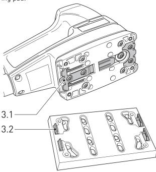
To ensure a better grip of the sanding pad on the sanding base of the LS 130 EQ you can fasten the sanding pad in the four holes in the corners (1.7) using the enclosed screws. These screws have to be removed before exchanging sanding pads.
