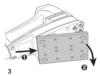
The new sanding pad is fitted in the reverse order. Make sure that the four lugs (3.1) of the sanding base catch in the four recesses (3.2) in the sanding pad.
