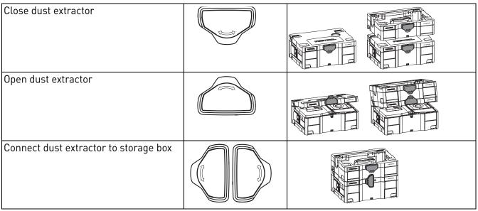
Before lifting, always close the T-Loc at the dust extractor or connect to the storage box and check for secure holding.
