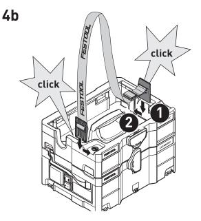
Before lifting, check the carrying strap for proper functionality and put T-loc at dust extractor into corresponding position.
