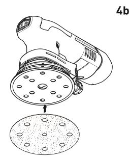
In the case of a weakening adhesive effect of the StickFix surface, the sanding pad accessories, in particular those which are not yet touching the workpiece, **may come loose from the sand**- **ing pad and cause injuries**. Replace the sanding pad!
