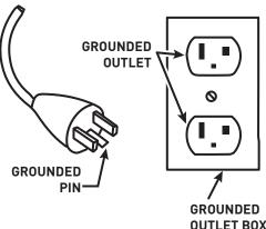
one way. If the plug does not fit fully in the outlet, reverse the plug. If it still does not fit, contact a qualified electrician to install the proper outlet. Do not change the plug in any way.
