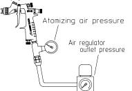
The gun should be held so that it is perpendicular to the surface of the work piece at all times. Then, the gun should move in a straight and horizontal line. Arcing the gun causes uneven painting.
