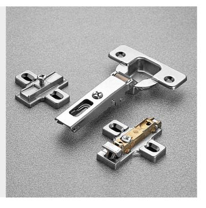
For thicker doors, max. 35 mm, with special profiles. 11 mm deep metal cup. 94° opening. Possible drilling distance on the door (K): from 3 to 9 mm. Compatible with all traditional Series 200 mounting plates and with
