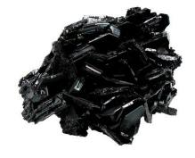
Silicon Carbide is a hard F, mineral, yet fractures easily to provide a sharp edge
