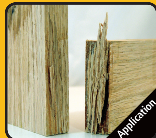
Breaks the wood, not the glue
