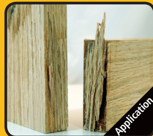
Breaks the wood, not the glue
