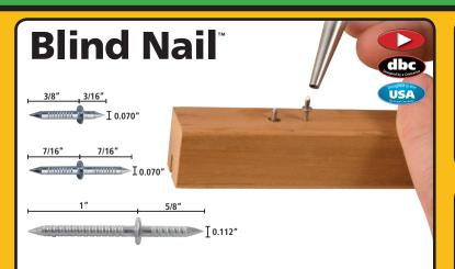
The Blind Nail allows you to have an invisible mechanical connector. Simply insert the dual head nail into the set tool to set the nail, then tap the molding or wood into place on the other side.
