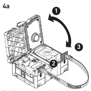
Carrying storage box with dust extractor: Carrying strap at storage box [4b]
