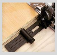
With an adjustable fence angle, retractable stops and adjustable cutter height with step gauge, the Domino joiner enables mortise placement and spacing. (Optional Cross Stop shown for illustrative purposes.)
