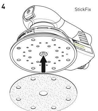
In the case of a weakening adhesive effect of the StickFix surface, the sanding pad accessories, in particular those which are not yet touching the workpiece, may come loose from the sanding pad and cause injuries. Replace the sanding pad!
