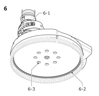
(i) If the machine cannot be started directly with a new sanding pad, rotate the sanding pad a few times by hand and run in.
