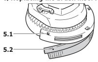
In order to replace this, press out the brush insert by inserting a screwdriver through the square apertures (5.1). Insert the new brush strip (5.2) into the groove, slightly bend this to obtain the correct radius and press in firmly until the brush strip is in contact with the base of the hood. The inclination of the brush bristles must point outwards.
