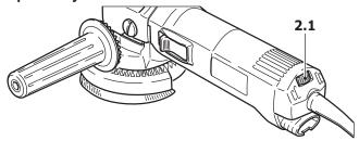
You can regulate the speed steplessly between 1500 and 4000 rpm using the adjusting wheel (2.1). This lets you optimize the sanding speed to suit the material (see "Working with the tool").
