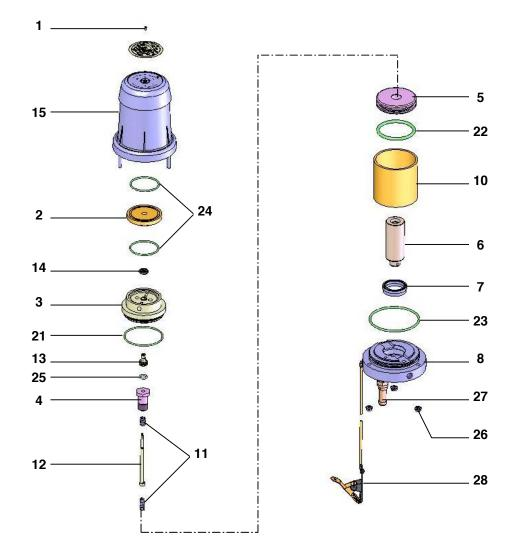
Disassemble the cover (15) by removing the 3 M6 screws (26).
