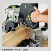
Rivaling most 12" saws 4-3/4" in its special cutting position, and 6-5/8" crown in the nested position. Can cut miters from 50° (left) to 60° (right).
