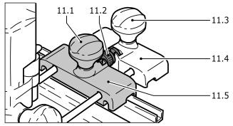
The distance X (fig. 10) of the router to the guide rail can be set finely using the fine adjustment (Accessories).
