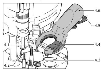
Chips and dust from routing can be removed by means of a extractor hood. See-through plastic material gives good view of rotating tool. You can connect a Festool extractor with an extractor hose diameter of 36 mm or 27 mm to the extractor connector (4.6). We recommend a diameter of 36 mm because it minimises the risk of blockages.
