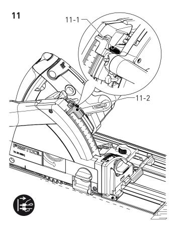
The cutting depth of resharpened saw blades can be adjusted accurately using the adjusting screw **[11-1]**.
