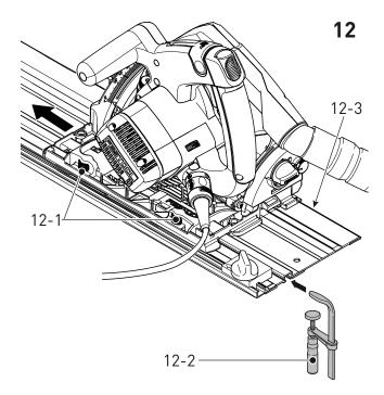
The splinterquard needs to be replaced if it becomes damaged or worn:
