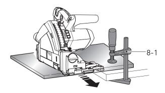
Ensure that your workpieces are securely fixed and cannot move during sawing. Otherwise, there is an increased risk of accident. Never hold the workpiece to be cut with your hands or between your legs. Use instead screw clamps **[8-1]** or some other suitable devices to fix your workpiece.
